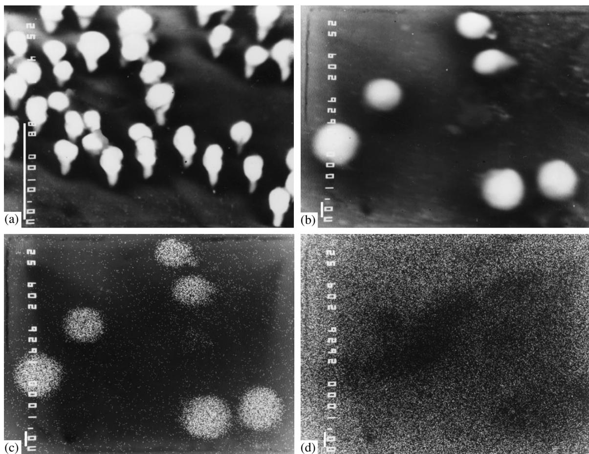
**Fig. 3.** Distribution of elements in metallic particles at the surface of the oxide shell; (a) and (b) surface element; (c) distribution of Ni; (d) distribution of Al in particles. (a) 4000 $\times$ ; (b), (c), and (d) 6000 $\times$ .
