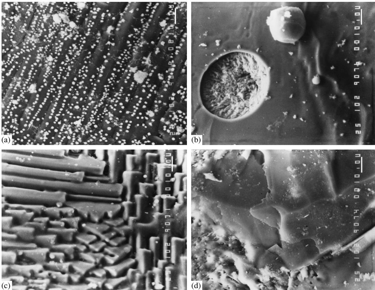
**Fig. 2.** Effect of microgravity on the microstructure of cast combustion products: (a) and (b) space experiments; (c) and (d) terrestrial experiments; (a) inner surface of the oxide shell; (b) outer surface of the oxide shell; (c) free surface; (d) surface adjacent to the metallic ingot. 400 $\times$ .
