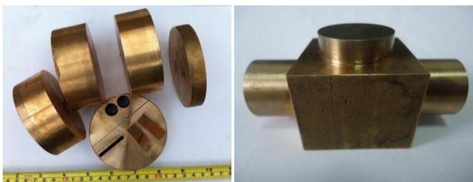
Figure 1. W-Cu materials prepared by combustion synthesis and centrifugal infiltration
