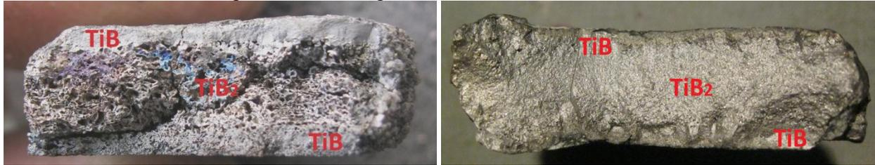
Fig.1. Macrostructure of the functionally graded material
