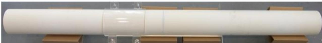
Fig. 2 SHS-joining of  $\text{Al}_2\text{O}_3$  pipes with 160 mm in diameter and 2,000 mm in length
