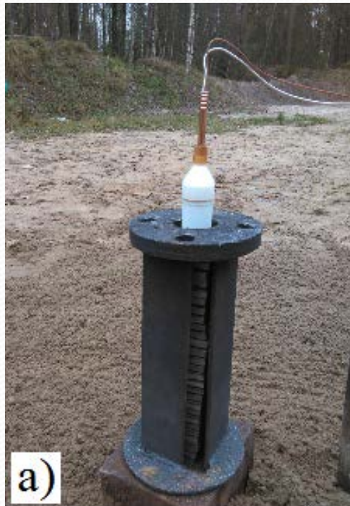
Fig. 4. View of prepared setup for control test of shaped charge (a) and view of plates after control test (b).
