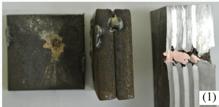
Fig. 7. Cumulative jet action towards 10 mm Ti layer
