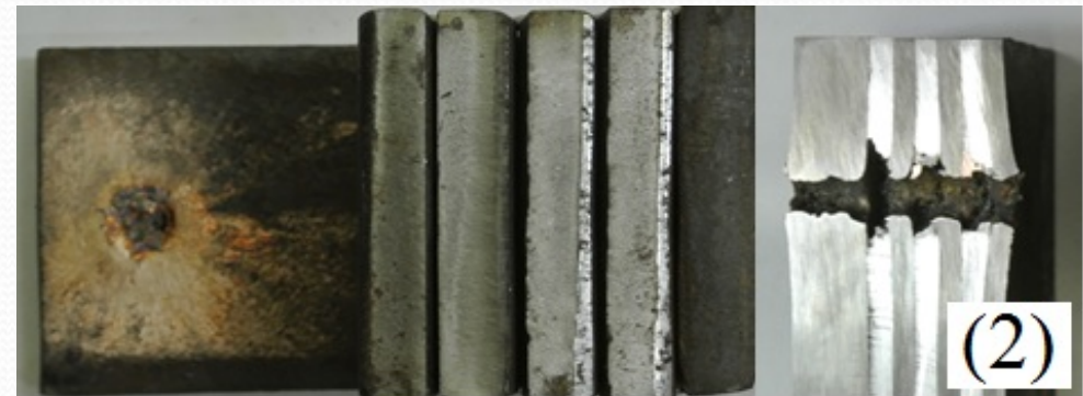
Fig. 8. Cumulative jet action towards 3 mm Ti layer
