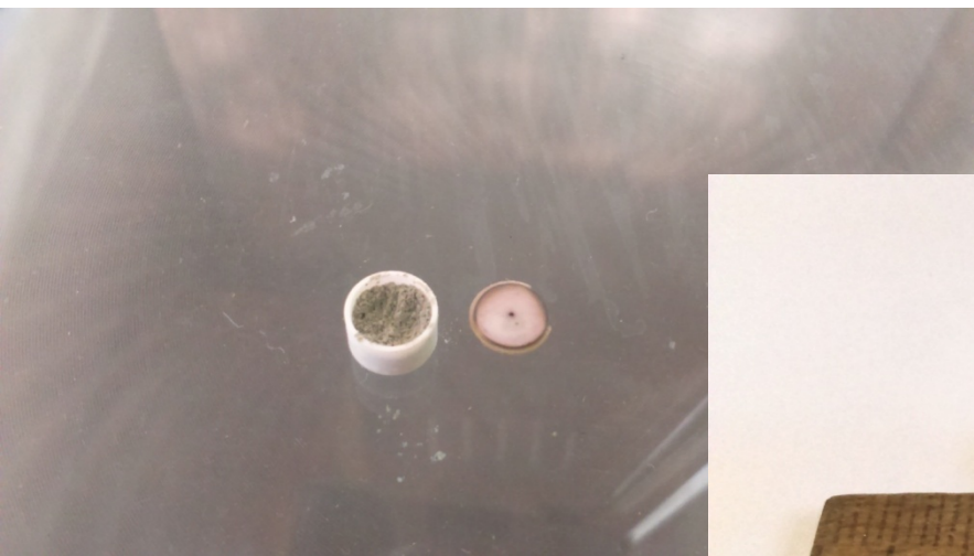
The crucible with the sample of detonation nanodiamond
