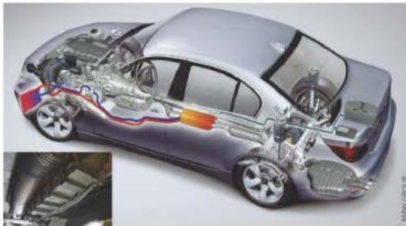
A car with thermoelectric waste heat recovery system BMW
