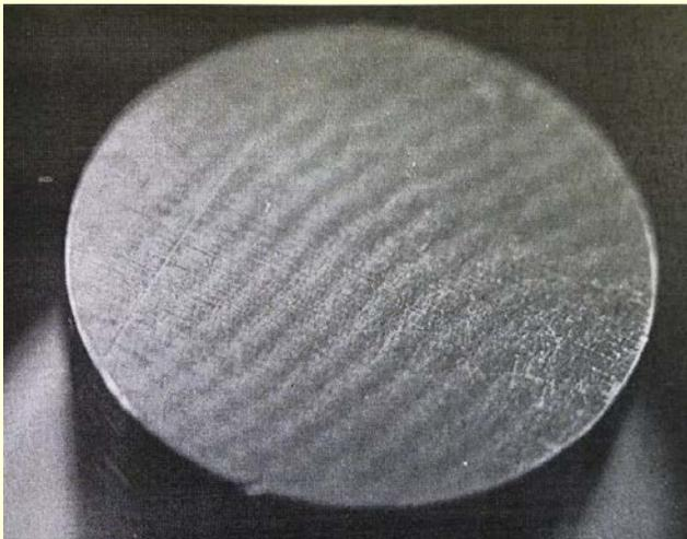
Waves on the steel-aluminum boundary
