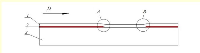
**Conclusion: The jet of copper particles provides formation of the strong bond between the plates of a high-strength steel in the low-speed collision mode.**
