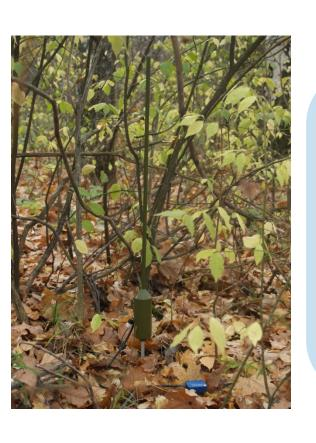
Total length of border up to 1,0 km **Total amount of participants** up to 50 Length of one sector from 3 to 20 m **Amount of participants' groups** up to 7 Period of unfolding of one not more than 5 min sector Period of continuous work not less than 80 days With seismic detector not less than 160 day Weight of the item in the operational packing (bag), not more than 7 kg
