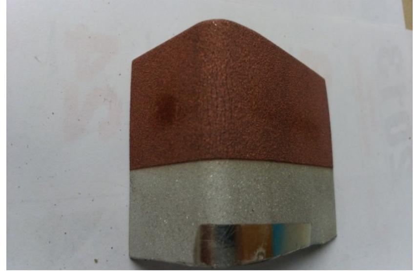
Cu coating on the Al alloy after bend test
