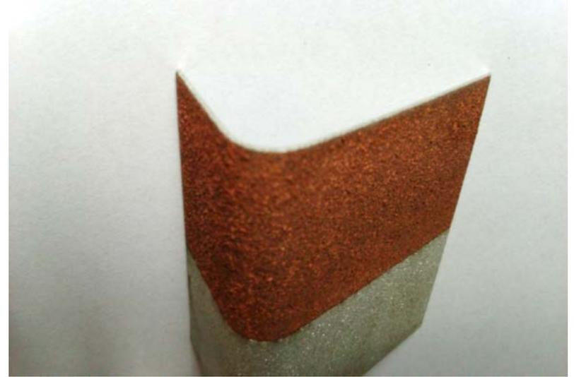
Cu-C coating on the Al alloy after bend test
