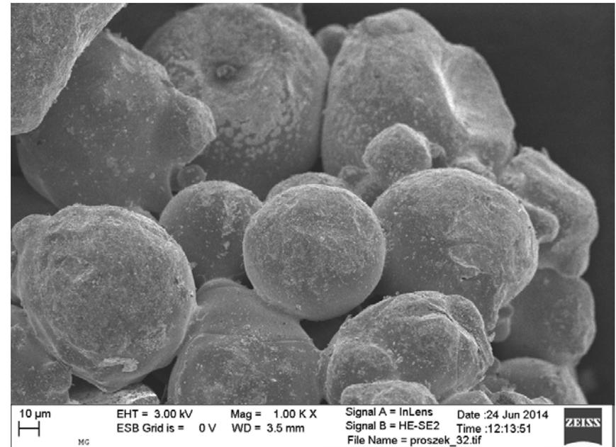
Spherical copper powder particles after graphene processing
