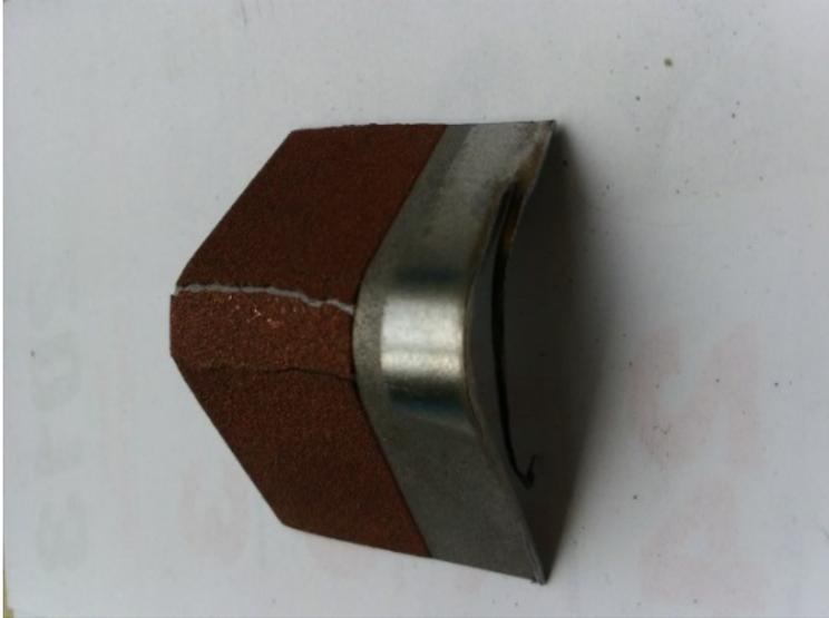
Cu coating on the S235JR steel after bend test
