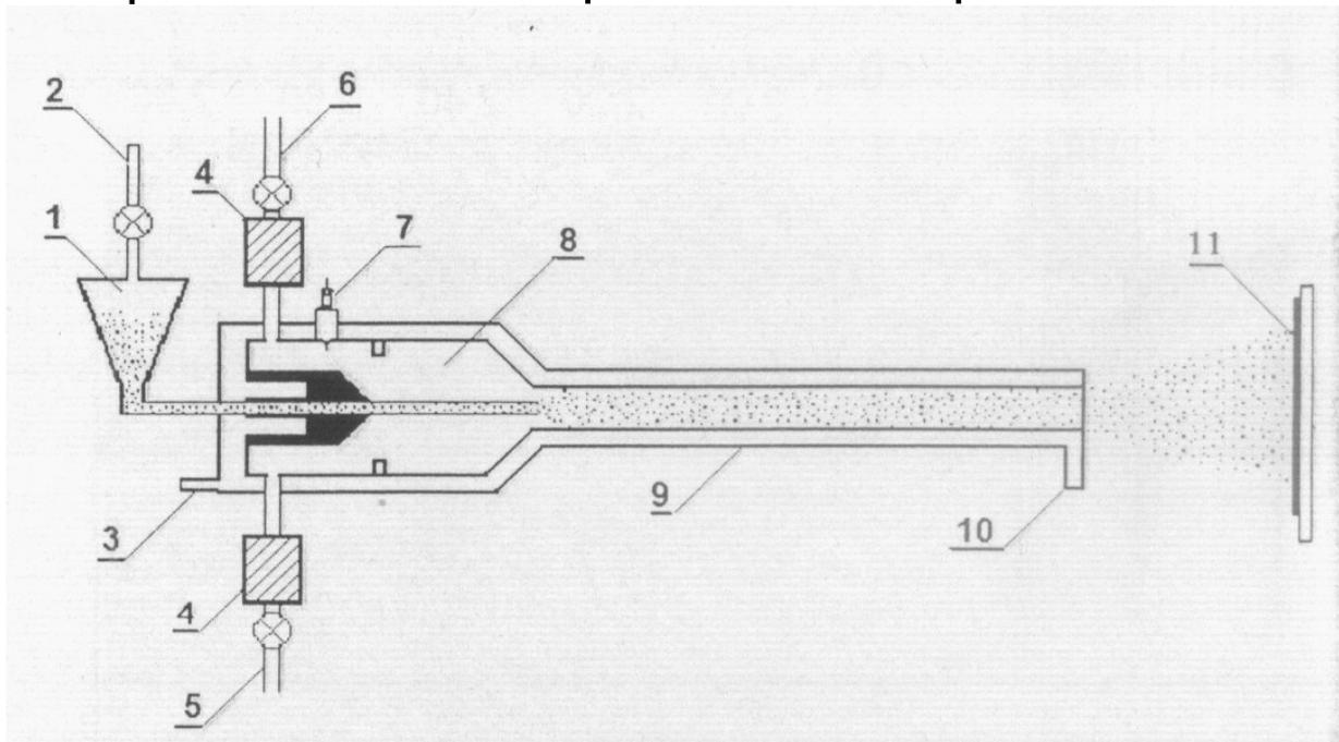
1- powder feeder; 2 – nitrogen; 3,10 – cooling system;
