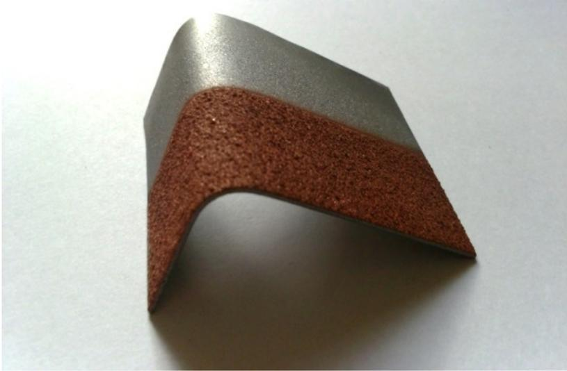
Cu-C coating on the S235JR steel after bend test
