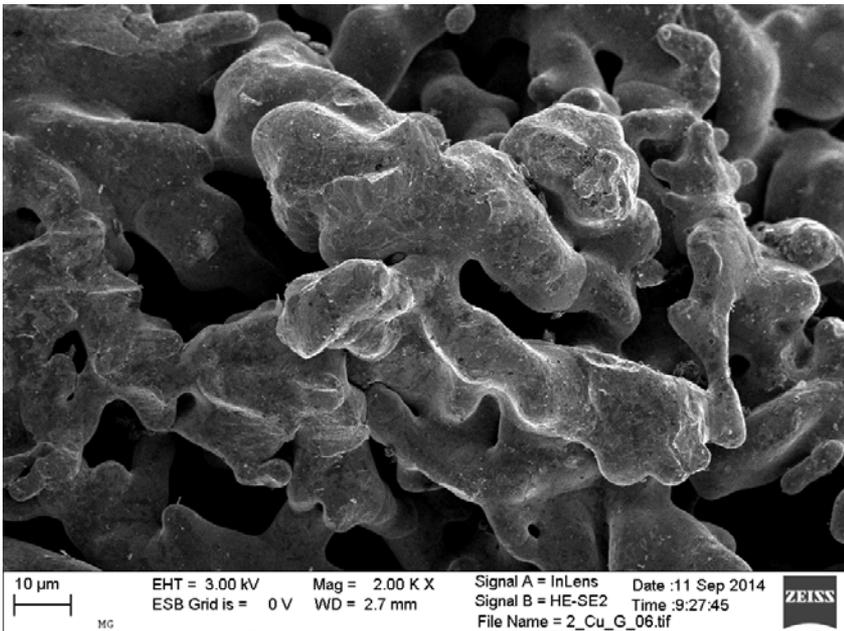
Dendritic copper powder particles after graphene processing
