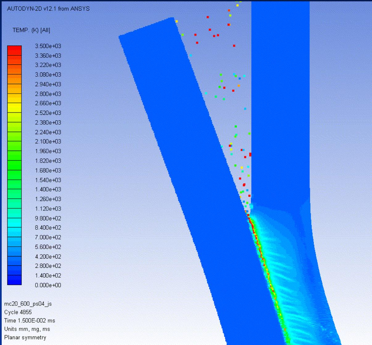
**Temperature was increased at over 3500 K in the interface of metals. The heat affected area was widened compared with the case of the Cu/Cu collision.**
