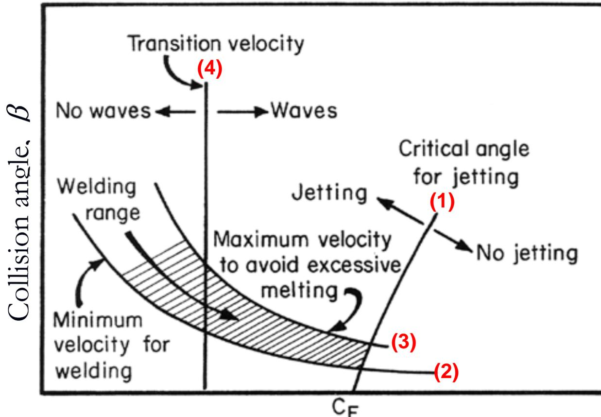
Horizontal collision point velocity,  $V_c$
