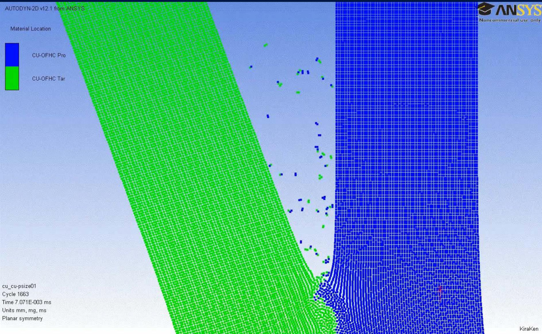
The metal jet consists of projectile and the target metal
