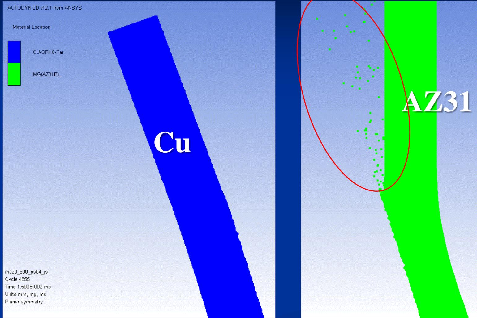
**The metal jet only consists of the projectile metal, AZ31 in Mg/Cu combination.**
