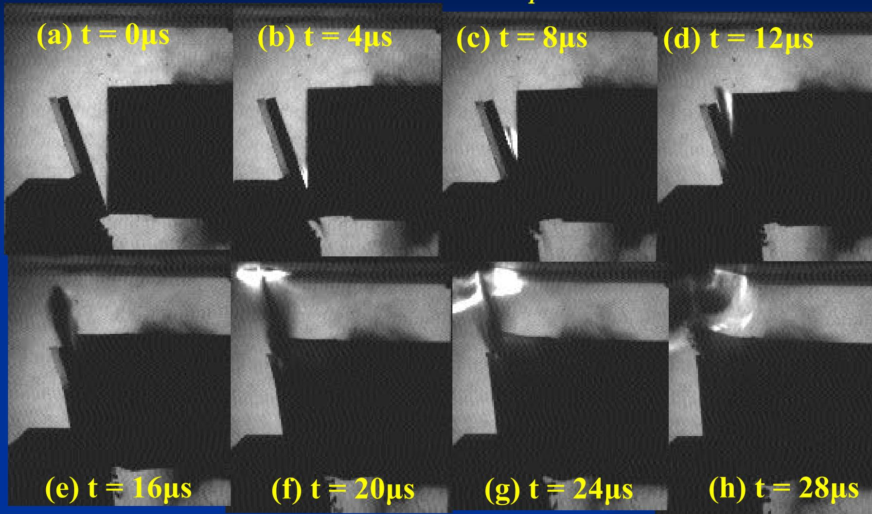
Collision point velocity :  $1670\text{ m/s}$  calculated by  $V_p = 2V_c \sin(\beta/2)$
