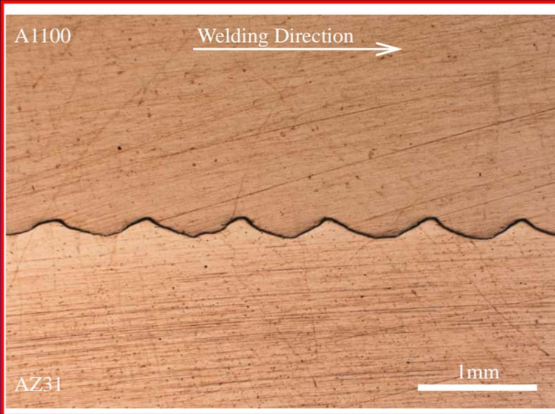
**Wavy interface of aluminum alloy / magnesium alloy**
