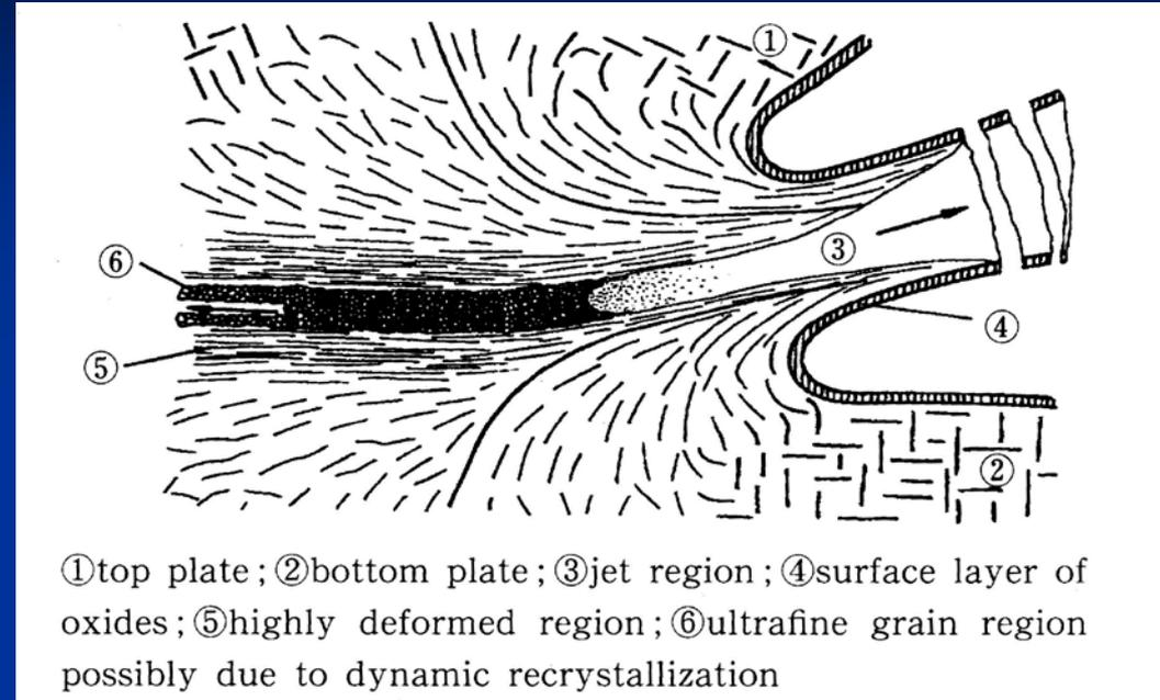
**Schematic of the metal jet generation**
