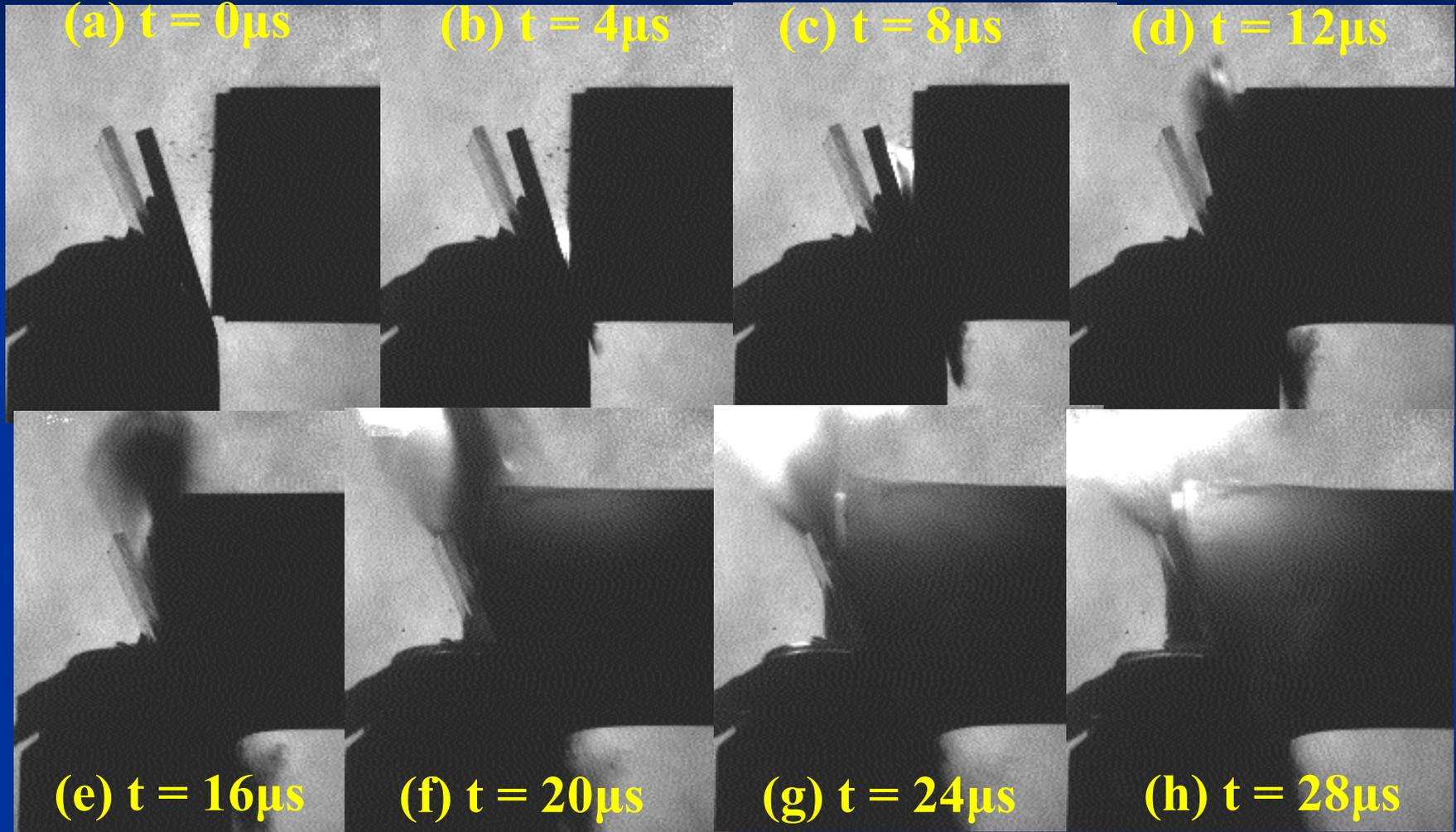
Collision point velocity :  $1756\text{ m/s}$  calculated by  $V_p = 2V_c \sin(\beta/2)$
