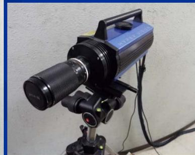
High-speed video camera, HPV-1 (Shimadzu Inc.)
