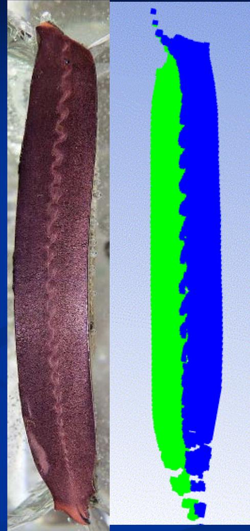
Velocity of the metal jet and the tendency of wavy interface generation are agree well with the experimental results.
