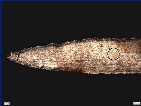
Cu-jet from interrupted cladding
