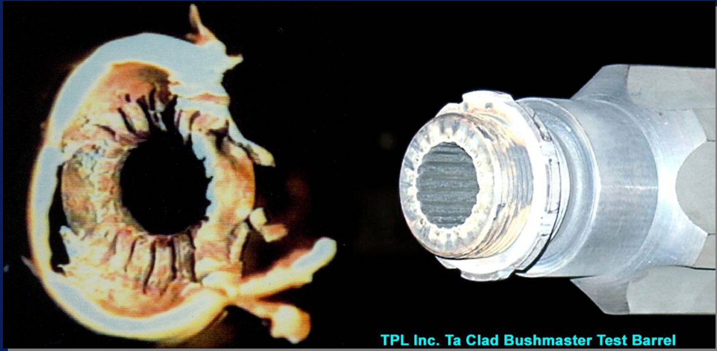
Ta-clad Bushmaster barrel after 600 shots (still serviceable)
