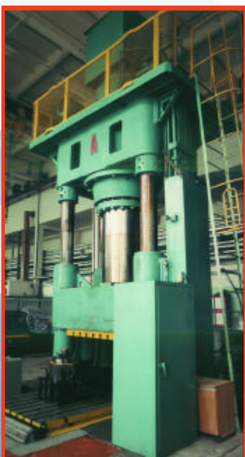
Press installation for obtaining large sized items by SHS compaction
