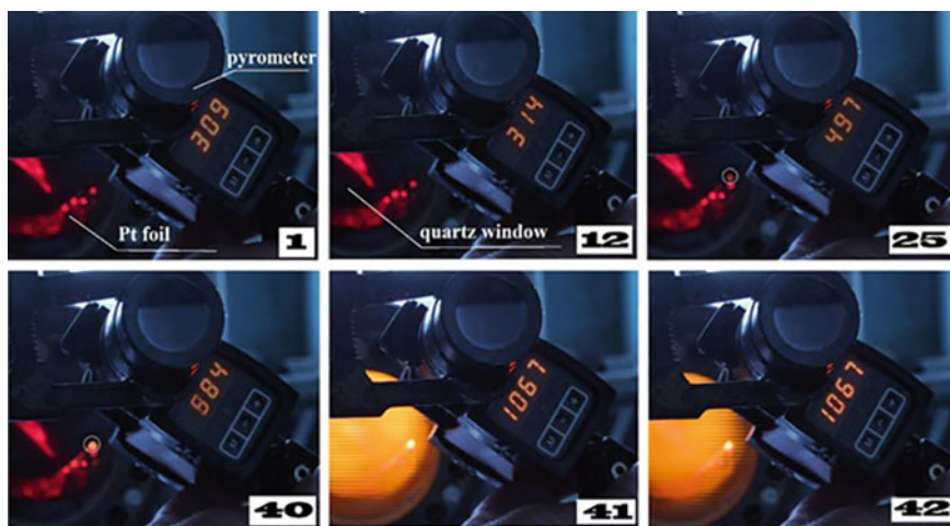
Fig. 2.26 Registration of the initiation of ignition of 40% H 2 + air with Pt foil with a two-beam color pyrometer indicating temperature values in °C. An ignition center on the foil is shown with a white circle in the frames 25, 40. P 0 = 1 atm. T 0 = 305 °C
