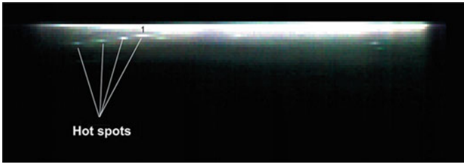
Fig. 2.14 RGB hyperspectral image of the combustion of a mixture of 40% H_2 -air, initiated by a platinum wire, obtained using a modified VID-IK3 hyperspectrometer, T_0 = 320 °C, P_0 = 1 atm, spectral interval 550–650 nm
