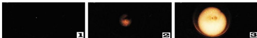
Fig. 4.4 High-speed filming of the catalytic ignition of the mixture 40% \text{H}_2 + air over Rh wire, 600 \text{ s}^{-1} , T_0 = 80 \text{ }^\circ\text{C} , P_0 = 1.7 \text{ atm} . The first number of the frame corresponds to the moment of the occurrence of a primary ignition center on the wire
