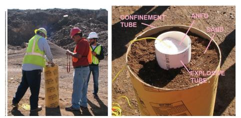
Fig. 1. Shockwave consolidation setup.
