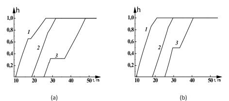
Fig. 1. Evolution in extent of conversion h at the upper (1), middle (2), and lower (3) part of the ampoule for mix I (a) and mix II (b).
