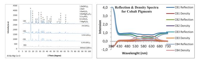
**Fig. 1.** XRD patterns of the samples:EB3 (Al-Ba-Mg-O),CB1 (Al-Ba-Mg-0,1%Co-O),CB2 (Al-Ba-Mg-0,5%Co-O), CB3 (Al-Ba-Mg-1,0%Co-O) synthesized through the solution combustion synthesis by heating at 600°C with the use of urea.
