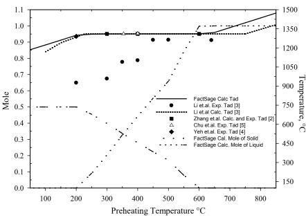
Figure 1 : The solid and liquid amounts in NiTi and the adiabatic temperature (Tad) values corresponding to the preheating temperature
