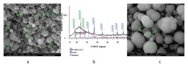
Figure 1. SEM images and diffraction patterns of metal oxide particles are obtained by solution combustion method: a, b)  $Co_3O_4$ ; c)  $CeO_2$
