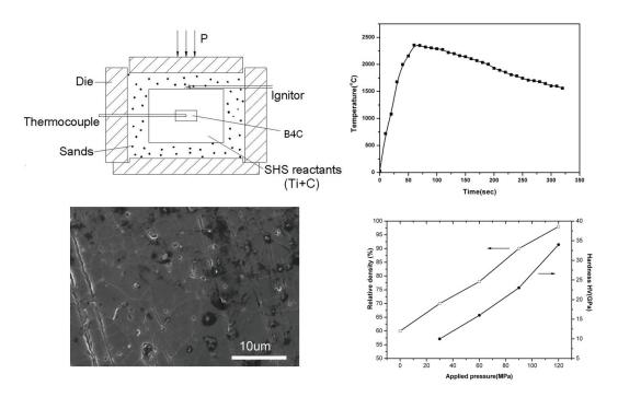
The B<sub>4</sub>C was densified by the heat from SHS with a heating rate of  $2300 \,^{\circ}$ C/min, and the mechanical pressure of 120 MPa in two minutes. The maximum hardness of the dense B<sub>4</sub>C specimen is  $34\pm0.2$  Gpa. This method has higher heating rate and shorter sintering time than traditional sintering process, which leads to maximal temperature and minimal grains coarsening.
