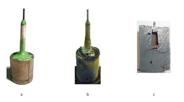
Fig. 2. Overall view of samples: (a) unburned, (b) burned, and (c) burned sample in cross section.
