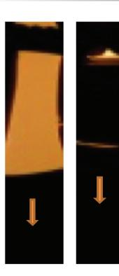
Figure 1. High-speed video frames of the SHS wave propagation in the Ni/Al multilayer reactive nanofoil: left - free standing Ni/Al reactive multilayer nanofoil, two-stage wave; right - the same on the Cu substrate, propagates only the first stage. (recording rate 40000 frames per second).
