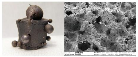
Fig.1. Burnt sample and microstructure of the product derived from Ni-Al mix containing 10% Cr<sub>2</sub>O<sub>2</sub>.
