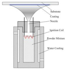
Fig.1.The device to prepare the  $Al_{2}O_{3}/ZrO_{2}$  eutectic coating by combustion-assisted thermal explosion spraying
