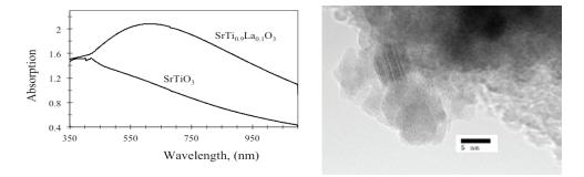
Figure 1. (left) The absorption wavelength spectra of SrTiO3 and SrTiO.9La0.1O3; (right) TEM image of SrTiO.9La0.1O3 nanoparticles, (bar-scale is 5 nm).
