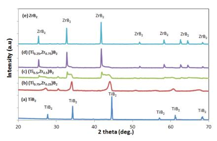
Fig.1 XRD patterns of (a)  $TiB_{2}$ , (b)  $(Ti_{0.75}$ ,  $Zr_{0.25}$ ) $B_{2}$ , (c)  $(Ti_{0.5}$ ,  $Zr_{0.5}$ ) $B_{2}$ , (d)  $(Ti_{0.25}$ ,  $Zr_{0.75}$ ) $B_{2}$ , (e)  $ZrB_{2}$
