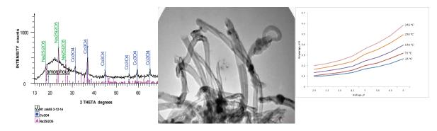
Fig. 1. a) X-ray analysis of glass fibers with nanoparticles of  $Co_3O_4$ ; b) TEM image of carbon nanotubes grown on glass fiber fabrics with  $Co_3O_4$  (5 wt. %); c) current-voltage characteristics of "array" of CNT grown on glass fiber fabrics with  $Co_3O_4$  (5 wt. %) at different temperatures
