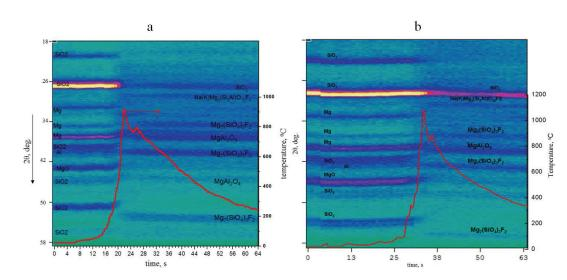
Figure 1. Diffraction pattern for mixture of 92% (SiO<sub>2</sub>-Mg-Al-Na<sub>3</sub>AlF<sub>6</sub>-KClO<sub>4</sub>)+8%MgO (a) and 85% (SiO<sub>2</sub>-Mg-Al-Na<sub>3</sub>AlF<sub>6</sub>-KClO<sub>4</sub>)+15%MgO (b).
