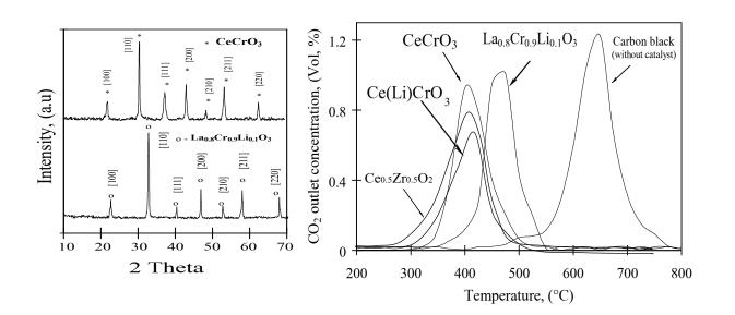
Figure 1. (left) X-ray diffraction patterns of as-synthesized CeCrO<sub>3</sub> and  $La_{0.8}Cr_{0.9}Li_{0.1}O_3$  produce by CCSO; (right) TPC runs of the catalytic carbon combustion over CeCrO<sub>3</sub>, Li-doped CeCrO<sub>3</sub>,  $La_{0.8}Cr_{0.9}Li_{0.1}O_3$  and  $Ce_{0.5}Zr_{0.5}O_2$  catalysts powder. Non-catalytic combustion of soot reported as a reference.
