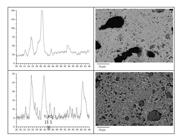
Fig. 1. A selected series of dynamic XRD patterns of combust sample at X = 20 % (a-c) and microstructures of SCF in different zones of combustion wave: d - initial mixture; e - post combustion zone; f - final product.
