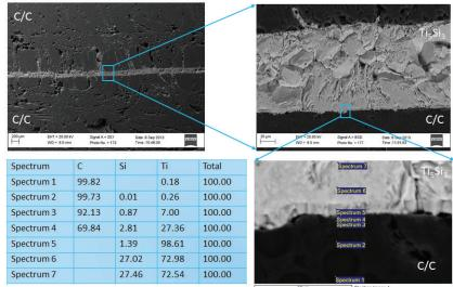
Figure 1. Typical SEM image of C/C composite joined with reactive ribbon of Ti+0.6Si.
