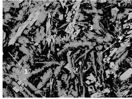
Figure 1. Back scattered electron microscopy image (×500) of hard alloy containing Mo<sub>2</sub>NiB<sub>2</sub> produced by SHS method (1: Ni<sub>3</sub>Al, 2: Mo<sub>2</sub>NiB<sub>2</sub>, 3: MoB)
