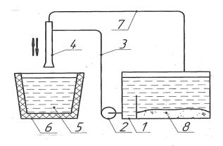
Fig.1. Device of molten granulation for obtaining the powder materials for SHS
