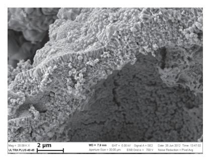
Fig. 1. Nano-structured particle of titanium nitride.
