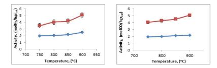
Figure 3: Activity (mol/hgrcat) H2 and CO by SCS catalysts in the systems Co-Al -O (60% Co(NO3)2-Al(NO3)3-urea-♦curves, 30% Co(NO3)2-Al(NO3)3-urea - ■curves)
