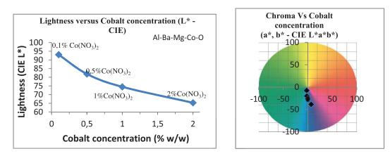
**Fig.3**. Lightness for Al-Ba-Mg-Co iluminascent pigments. CB1 sample precursor contains 0,1% Co, CB2 sample precursor contains 0,5% Co, CB3 sample precursor contains 1,0% Co and CB4 sample precursor contains 2,0% Co.
