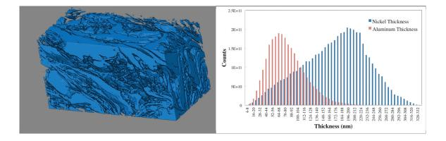
Figure 1: a) 3D reconstruction of Ni/Al composite particle, b) Layer thickness distribution obtained with 3D reconstruction.
