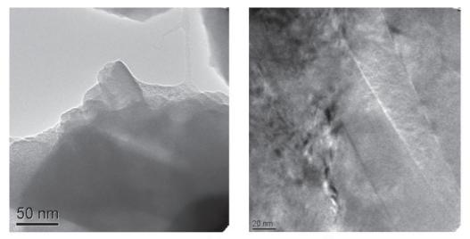
Fig. 1 TEM images of Ti<sub>2</sub>SC phase; (a) thin film-like and (b) band-like structures.
