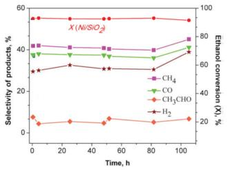
Figure 1: Conversion (X(Ni/SiO<sub>2</sub>)) and selectivity of methane, carbon monoxide, hydrogen, and acetaldehyde during the ethanol decomposition over Ni/SiO<sub>2</sub> catalyst, 200 °C.
