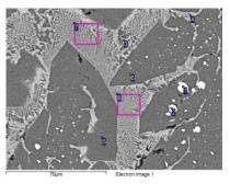
(a) (b) Fig. 1. The microstructure of the metal (a) oxide and (b) layers. The initial mixture  $Ti/Al/CaO_2/Nb_2O_5/Cr_2O_3$ . Overloading a = 250g
