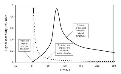
Fig.1 Dependencies of pressure variation rate in the chamber, and square of the acoustic emission signal amplitude on time of compact titanium hydrogenation
