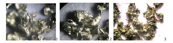
Fig.2. Microphotographs of the obtained powders, x100. 1-Al; 2-Al+Mg; 3-Fe;
