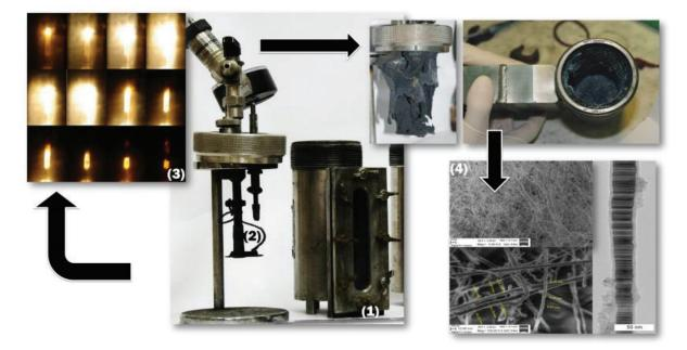
Experimental setup: high-pressure stainless-steel reactor with optical follow-up of the combustion (extremely fast process, within 1 s) and SEM/HR TEM images of products (SiCNFs with diameter 50 nm  $\pm$  20 nm and length up to several microns).
