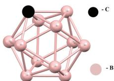
Fig.3. Icosahedral cell of boron carbide.
