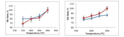
Figure 1: Conversion of CH4 and CO2 by SCS cobalt catalysts (60% Co(NO3)2-Al(NO3)3-urea-♦curves, 30% Co(NO3)2-Al(NO3)3-urea-♦curves)
