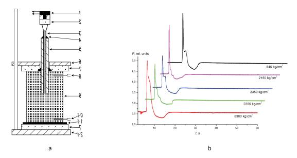
Fig. 1. (a) Experimental setup: 1, pressure gauge; 2, mineral wool; 3, syringe needle; 4, heat-resistant glue; 5, ceramic tube; 6, clamping plate; 7, BN plate; 8, thermocouple T2; 9, sample; 10, thermocouple T1; 11, initiating TiB strip; 12, bedding; and (b) typical pressure profiles recorded by gauge 1 (indicated are compacting pressures).
