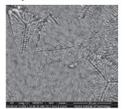
Fig.1 Backscattered electron image of Al<sub>2</sub>O<sub>3</sub>/ZrO<sub>2</sub> eutectic
