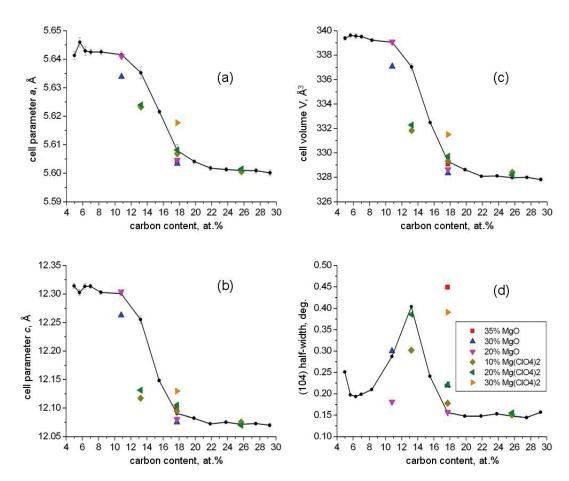
Figure 1. Cell parameters (a–c) and half-width of (104) reflection (d) for boron carbides synthesized at 2000°C in paper [1] (solid lines) and at 1500–2500°C (symbols).
