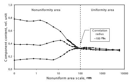
Fig.1. Example of correlation radius determination for two-component SHS composition
