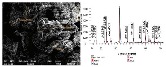
Fig. 1. SEM image of microstructure and XRD analysis of MgB,
