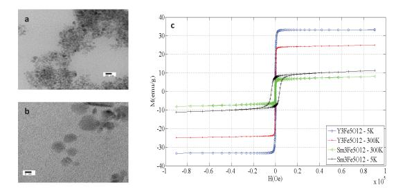
Figure 1. TEM images of yttrium ferrites produced at 3 wt. % glycine: the bar scale (a) - 20 nm; and (b) - 5 nm; (c)
