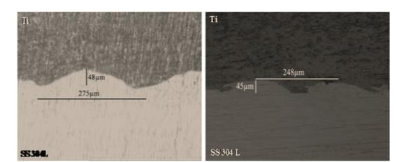
Fig.2. Microstructure of Ti-SS304L explosive clad
