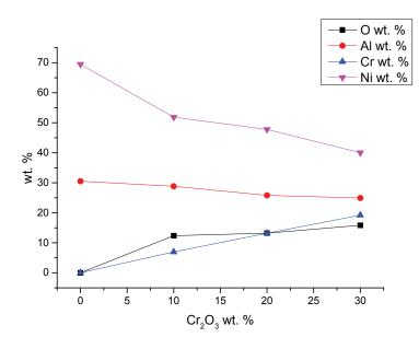
Fig.2. Chemical composition of the burnt  $Cr_2O_3$ -NiAl samples vs.  $Cr_2O_3$  % content.
