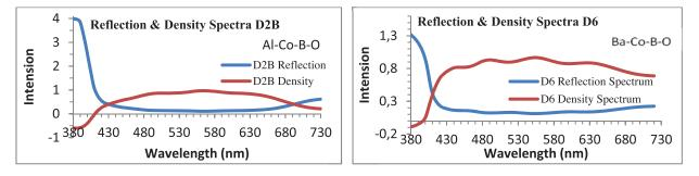
**Fig.7** Reflection and Density Spectra for Al-Co-B-O pigments pigments.
