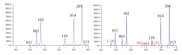
Fig. 2. Theoretical XRD patterns of B<sub>4</sub>C crystal modeled without (left) and with (right) account of icosahedron distortion.
