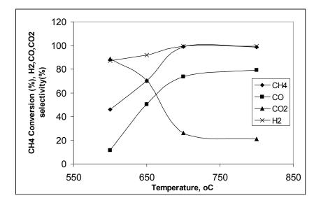
Fig.1 CH4 conversion and H<sub>2</sub>, CO, CO<sub>2</sub> selectivity over Co-Al-O SHS catalyst in partial methane conversion
