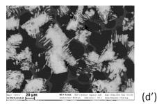
Fig.1. SEM images of alloy I: SHS-produced (a, a') and after remelting at 1700 (b,b'), 1750 (c, c') and 1800 °C(d, d').
