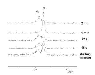
Fig. 1. Fragments of XRD pattern of powder mixture of the Nb - 62.3 mass. %, Si - 37.7 mass.% composition after various time MA.
