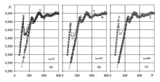
Fig.1. Relative density  $r_0$  of compact as a function of N ( $D_3$ =15mm): a) $\alpha$ =0°;  $\beta$ ) $\alpha$ =45°;  $\beta$ ) $\alpha$ =90°.
