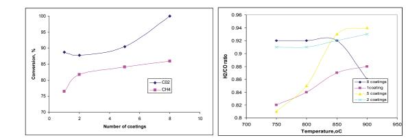
Fig1. Influence of number of coatings during preparation of catalysts on carrier (on the base of MgO-MgAl<sub>2</sub>O<sub>4</sub>) on conversion CH4, CO<sub>2</sub> and  $H_2$ /CO ratio.
