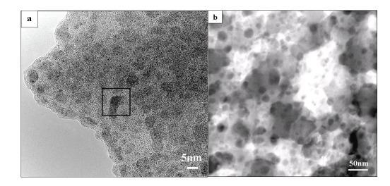
Fig.1. HRTEM images of Cu-Cr pseudo alloys formed at: (a) s = 60 min of HEBM, (b) s = 60 min of HEBM and SPS -consolidation at 700°C
