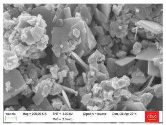
Fig. 1. SEM observation of a powder synthesized by mechano-chemistry
