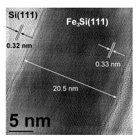
Fig.1 Cross-sectional HRTEM image of the Fe<sub>3</sub>Si/Si(111) structure.
