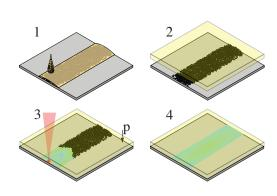
Fig. 1: Drawing of the concept: (1) Deposition of the nanocomposite dispersion. (2) Alignment of top substrate after solvent evaporation. (3) Ignition of SHS reaction while applying pressure. (4) Finished bond.
