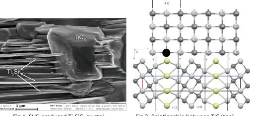
Fig.1. SHS-produced Ti<sub>3</sub>SiC<sub>2</sub> crystal. Fig.2. Relationship between TiC (top) and Ti<sub>3</sub>SiC<sub>2</sub> (up) structures: • stands for hole, distance in Å.
