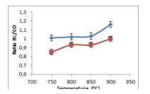
Figure 2: Ratio H2/CO by SCS catalysts in the systems Co-Al -O (60% Co(NO3)2-Al(NO3)3-urea-♦curves, 30% Co(NO3)2-Al(NO3)3-urea-♦curves)
