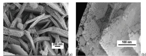
Fig. 1.SEM micrograph of Fe-based (a) catalyst surface for deep oxidation and (b) Co-Ce catalyst for FT process
