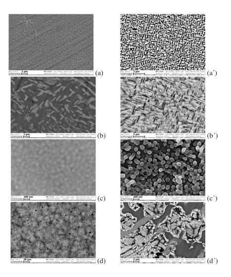
Fig. 1. SEM images of HEAs: polished (a, b, c, d) and after etching (a', b', c', d'); (a, a') NiCrCoFeAl, (b, b') NiCrCoFeAlCu, (c, c') NiCrCoFeMnAl<sub>16</sub>, (d, d') NbTiMoZrCrAl<sub>05</sub>Si<sub>10</sub>
