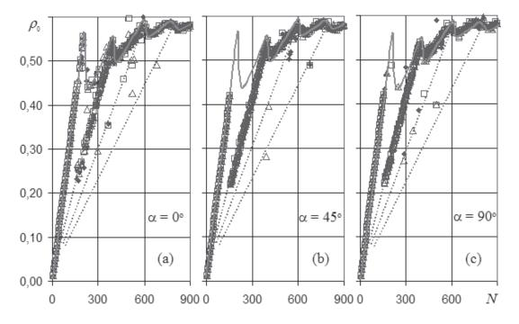
Fig.1. Relative density of the compact  $r_o$  as a function of N ( $D_3$  =15mm): a)  $\alpha$ =0°;  $\beta$ )  $\alpha$ =45°;  $\beta$ ) $\alpha$ =90°.
