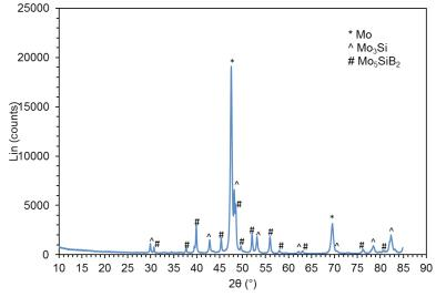
Figure 1: XRD pattern of products obtained by combustion of Mo-12Si-8.5B mixture.
