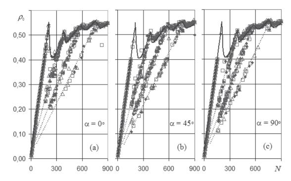
Fig.1.Relative density of the compact  $r_0$  as a function of N (L=14 MM): a) $\alpha=0^\circ$ ; $\beta\alpha=45^\circ$ ; $\beta\alpha=90^\circ$ .
