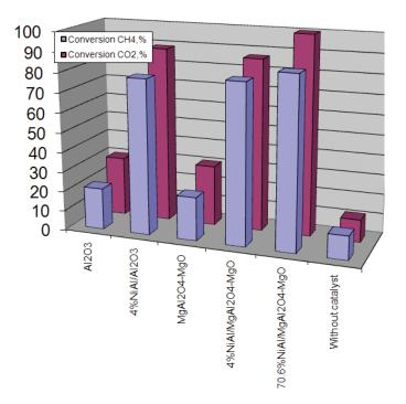
Fig.2. Influence of carrier on the catalytic activity of coatings produced by CAFSY method.
