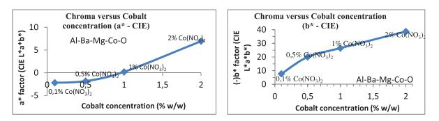
**Fig. 5** a\* factor - Red colour (CIE L\*a\*b\*) increases as the concentration of the Co increases in the precursor mixture from 0,1 to 2,0%
