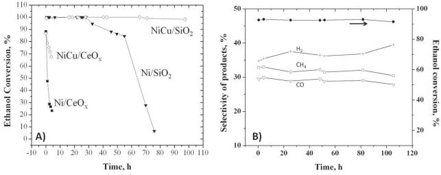
**Figure 1.** Ethanol conversion over A) standard SCS prepared single and bimetallic catalysts and B) Ni/SiO<sub>2</sub> prepared by SCS under 5 atm inert atmosphere
