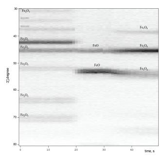
Fig. 1 The diffraction picture of the combustion process of mixture  $Fe_2O_2$  - hexogen.
