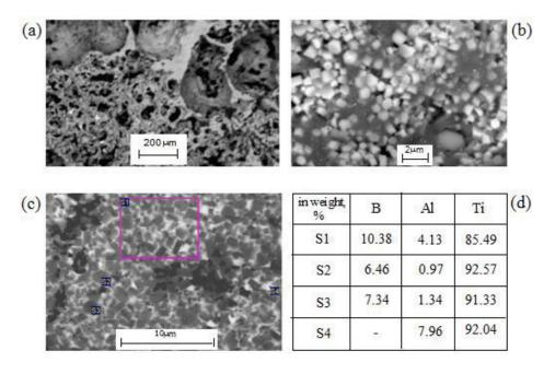
Fig.1. Synthesis product structure: a) macropores, b) macropore surface, c, d) material microstructure and elemental composition (*a*=0.8).
