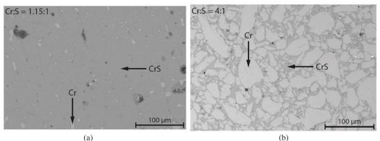
Figure 1: Micrographs of (a) Cr:S molar ratio 1.15:1 and (b) Cr:S molar ratio 4:1 cermets. The light gray phase is metallic chromium, while the darker matrix is chromium sulfide.
