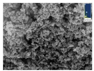
Fig 1 Morphology and EDX spectrums of nano-sized amorphous boron powder
