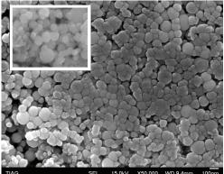
Fig. 2: SEM micrograph of a reacted AlTi sample. The initially spherical nanoparticles formed one layer comprising nonspherical grains. The insert shows the unreacted RNC layer.
