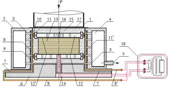
Fig.1. Design of the new press-mold for the electro-forced SHS compaction.
