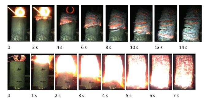
Fig. 1. Combustion propagation over compacted mixtures of (top) Mojave Mars and (bottom) JSC-Mars-1A regolith simulants with magnesium (20 wt% Mg). Time zero was selected arbitrarily.
