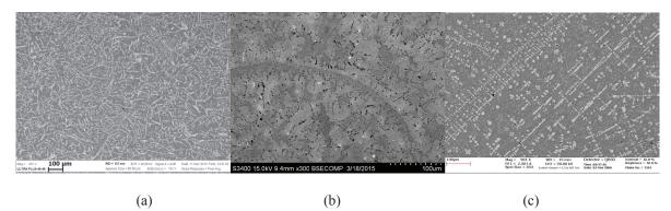
Fig. 1. The microstructure of SHS-produced CMs: (a) Ni-Mo-Al-Hf-Mn-B, (b) Ni-Al-Co-Cr-B), and (c) Co-Nb-Cr-W-Mo-Al-C.
