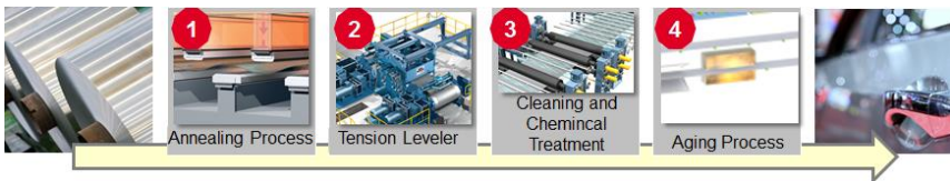
Fig.3 - Process route in a heat and chemical treatment line to produce HT alloys
