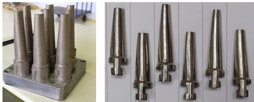
Fig. 2. SLM model of the blades of gas-turbine engine made of spherical CompoNiAl-M5-3 powders.
