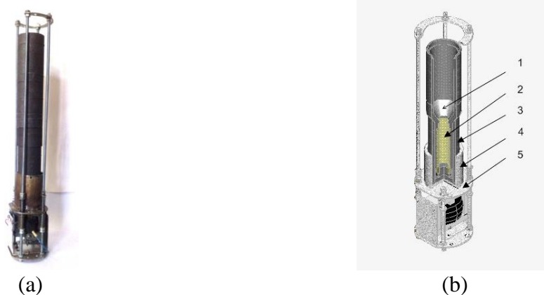
Fig. 2. Vibration installation: interior (a), drawing in 3D (b). 1 graphite adapter, 2 quartz forming tube, 3 graphite form, 4 protective glass, 5 vibrating table.
