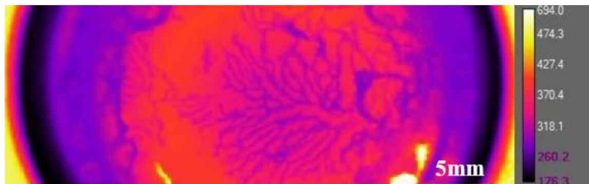
Fig. 1. Photograph of the sample during SCS, taken using an IR camera.
