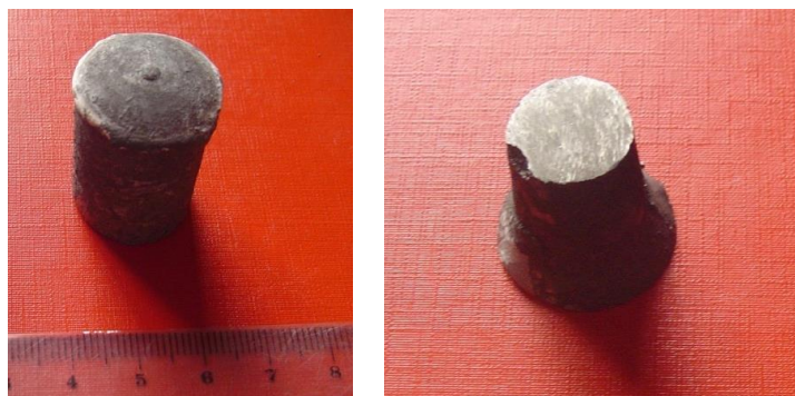
Fig. 1. The cast samples with various geometrical form with height of 45 mm received by laboratory centrifugal machine.
