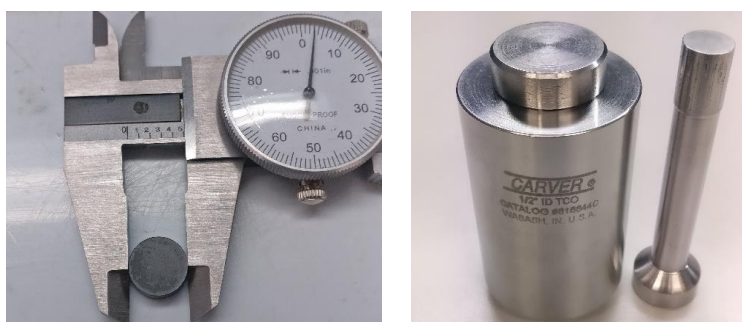
Fig. 1. As pressed pellet (left), punch and die (right).
