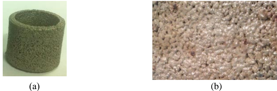
Fig. 3. (a) Experimental sample and (b) state of its surface after the generation of self-propagating high-temperature synthesis.
