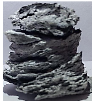
Fig. 4. Fracture and external appearance of SHS samples obtained with magnesium modified at MCT with a content of 20% C.
