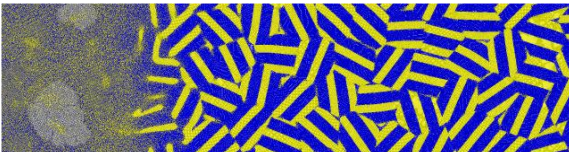
Fig. 3. Snapshot of SHS propagation in a sample with 80 disoriented 15 nm-grains. Each grain has a layered structure.
