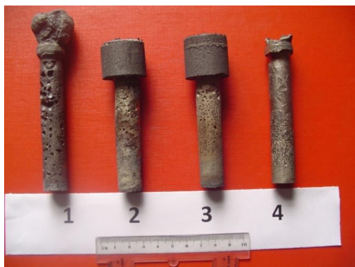
Fig. 5. The samples received in the high-pressure reactor as a result of vibration: 1 amplitude of fluctuations is 0.1 mm, frequency is 50 Hz; 2 amplitude of fluctuations is 0.2 mm, frequency is 100 Hz; 3 amplitude of fluctuations is 0.2 mm, frequency is 50 Hz; 4 amplitude of fluctuations is 0.1 mm, frequency is 100 Hz.
