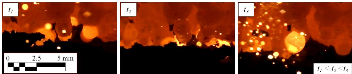
Fig. 4. Instantaneous time sequent photographs of the SHS process. The reaction mixture of (Ni + 20 wt % Al) + 2 wt % CaCO 3 .
