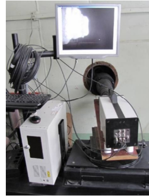
Fig. 2. The appearance of the camera NANOGATE-4BP.
