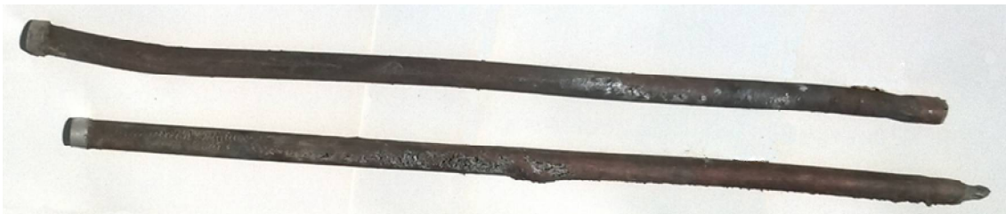
Fig. 2. Long-length coaxial billets after explosion welding: from above - with vacuum, from below - without vacuum; the direction of detonation from left to right.
