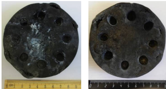
Fig. 2. Overall view of matrices after the shock-wave loadings of the initial (left) and mechanically activated (right) compositions.
