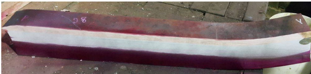
Fig. 4. The bimetallic blank tested by PT.
