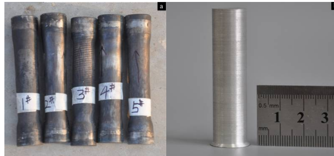
Fig. 1. (a) As recovered compacted containers with reduced diameter and (b) the specimen machined out from container.
