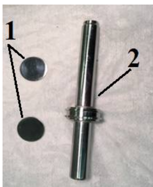
Fig. 3. (1) Sample-witnesses and (2) stock model with a protective coating including detonation nanodiamonds. Sputtering was carried out at Petrovsky Scientific Center FUGAS, JSC.
