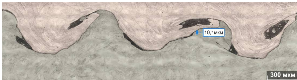
Fig. 2. The bimetallic interface
