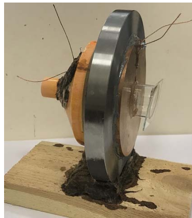
Fig. 4. Photo of experimental assembly (1 – sample of the fiber core)
