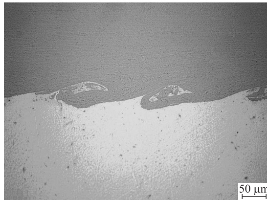
Figure 1 Microstructure of W clad (1 mm) onto Cu (5 mm)
